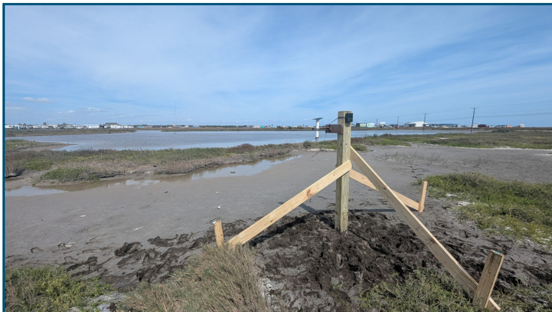
Figure 1. Photo of the Hohonu sensor when there is no water, at the site. Water can be seen further away in the wetland.
