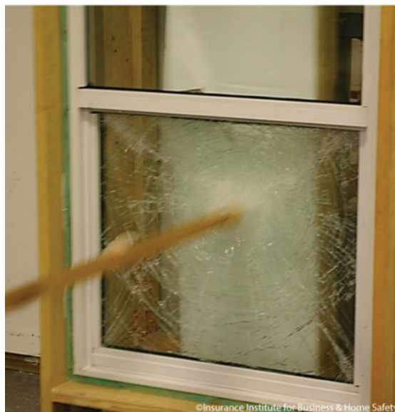
Figure 3-20. Impact Test on Window Source: FEMA
