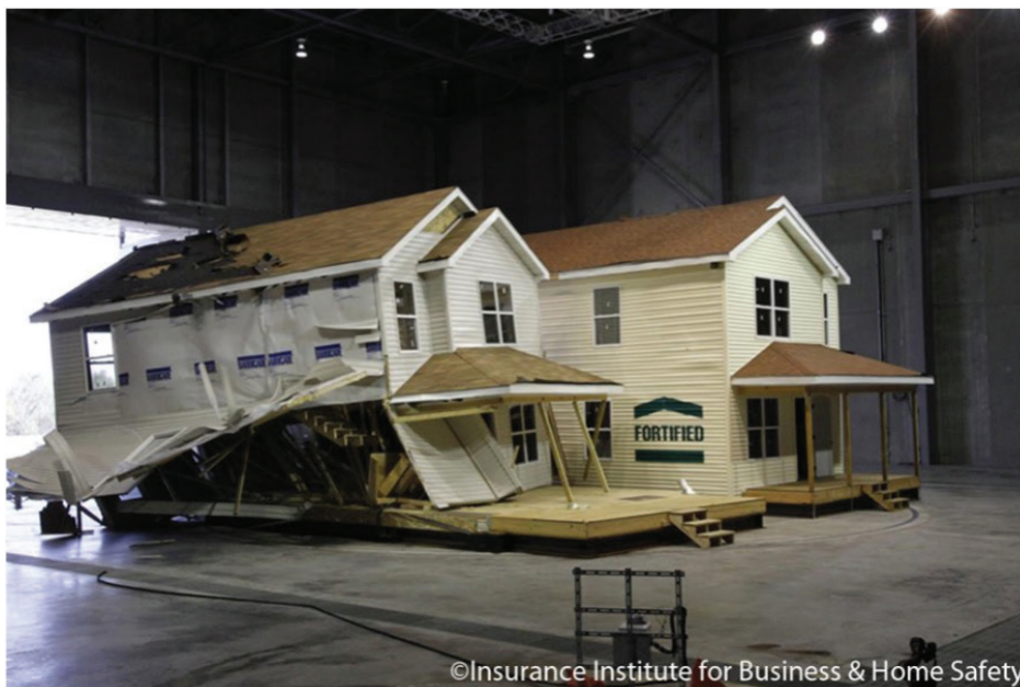
Figure 3-2. An IBHS FORTIFIED home (back) versus a home that was not built according to FORTIFIED standards (front) after being subjected to standard thunderstorm conditions Source: IBHS.
