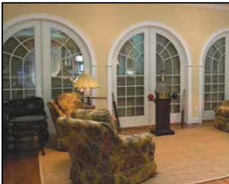
Figure 4-7. Interior of home with deployed roll-down shutters. Roll-down shutters can be used not only for storm protection, but also for security, privacy, light, heat, and noise control.
