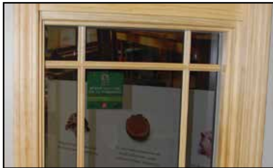
Figure 4-17. This attractive window can be fitted with energy-efficient glass, impact-resistant glass, or both. The impact-resistant glass consists of a laminate or film sandwiched between two glass panes. The frames are reinforced and the hinges have an extra fastener to withstand high winds. During a wind event, debris may crack the glass, but the laminate will hold the windowpane together in the frame and prevent breaching of the wind- and rain-resistant envelope. After the storm, the glass will need to be replaced.
