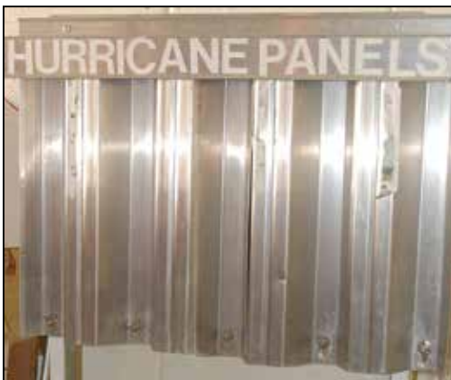
Figure 4-12. Although installation varies, this example shows panels that slip into a track above the window. The bottoms of the panels are secured by bolts that permanently attach to the window.
